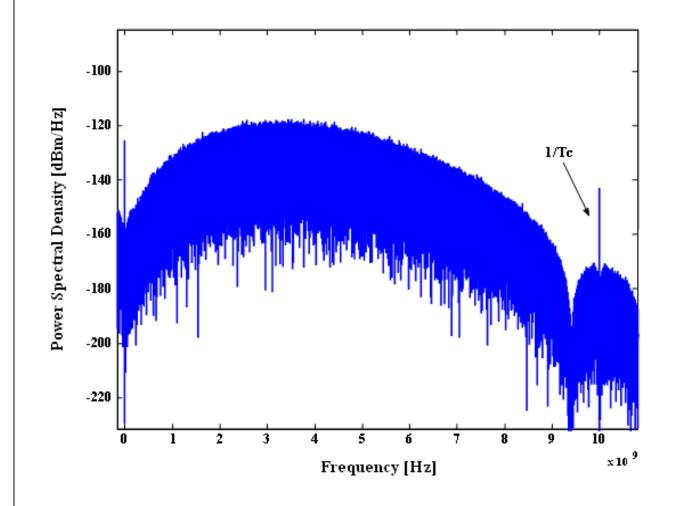
➢We now reduce the value of *Tc* to 0.1ns. As expected, the introduction of a quasi-fluid TH code has the effect of eliminating peaks in the PSD of the transmitted signal
