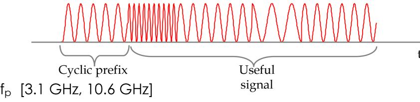
[3.1 GHz, 10.6 GHz] is divided into 13 frequency sub-bands (one for each MB-OFDM band):
