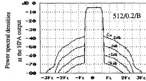
Fig. 4. Power spectral densities of the signal at the HPA output for various output back-off values ( C = 2, 0, -2, -4 dB, as indicated on the curves), and in the L = 512/\gamma = 0.2 /case B configuration.
