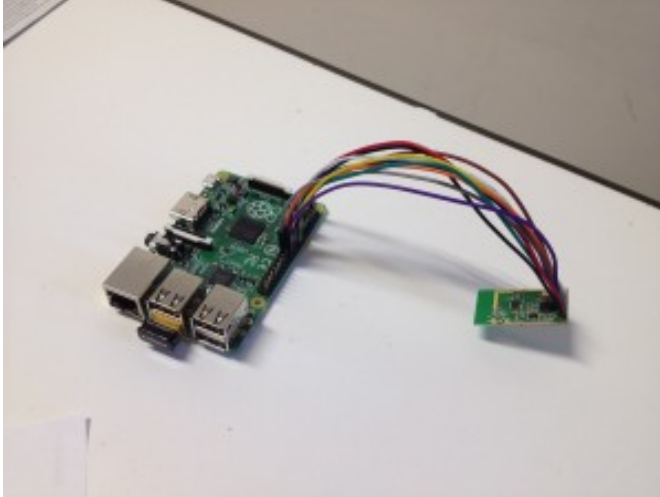
Figure 1. Network device in the WAN4RP demo platform, composed by a Raspberry Pi B+ connected to the RFM73P-S2 transceiver.
