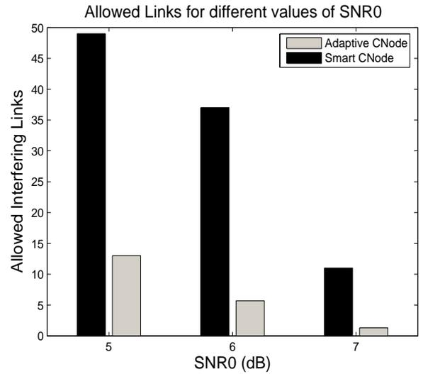
Fig. 5. Number of interfering links allowed by the Adaptive CNode and by the Smart CNode for different values of the synchronization threshold  $SNR_0$ .
