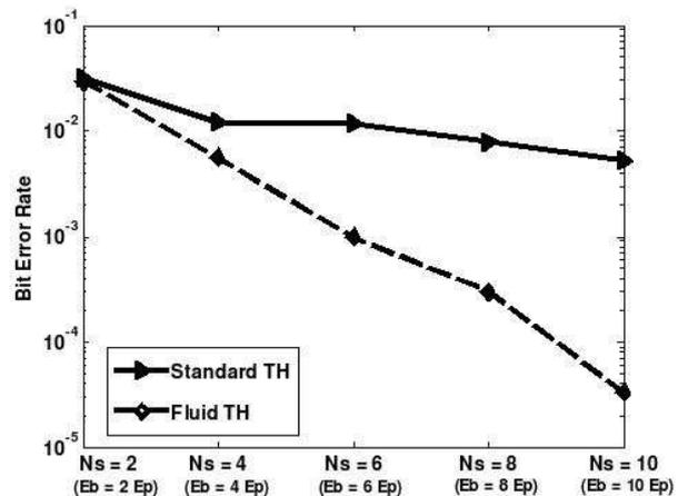
Fig. 9. BER in the two cases of standard TH coding (full line and triangles) and Fluid TH coding (dotted line and losanges) for the considered ring topology (radius = 10 m and 10 nodes) for different values of the number of pulses per bit  $N_s$ . The corresponding transmitted energy per bit  $E_b$  is also indicated for convenience as a multiple of the energy per pulse  $E_p = 1.49 \cdot 10^{-18}$  Joule
