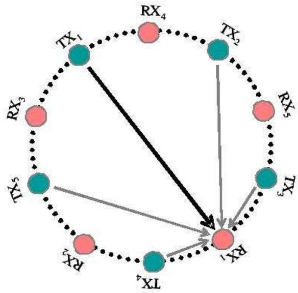
Fig. 8. Ring topology including 10 nodes: nodes are alternately transmitters and receivers. Each transmitter is associated to the receiver diametrically opposed.
