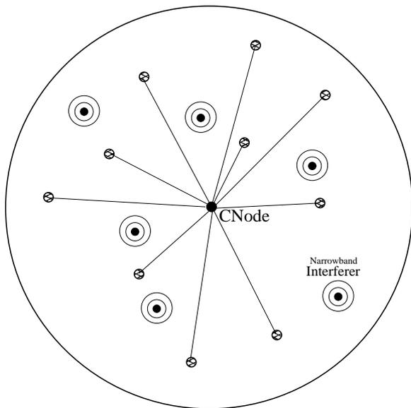
Fig. 1. The reference network, centralized in the CNode, faces the interference caused by narrowband transmitters become active in the area.
