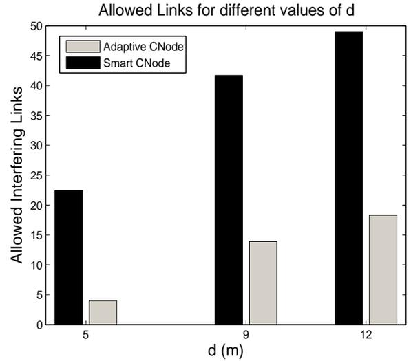
Fig. 6. Number of interfering links allowed by the Adaptive CNode and by the Smart CNode for different values of distance  $d$  between the CNode and the MNode.
