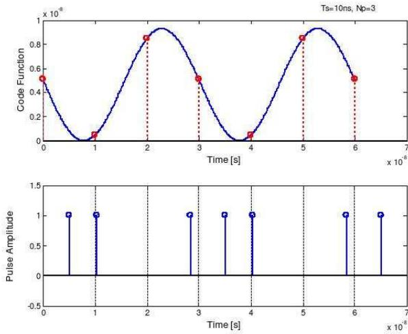
Fig. 7. Fluid Coding obtained sampling a sinusoidal waveform.
