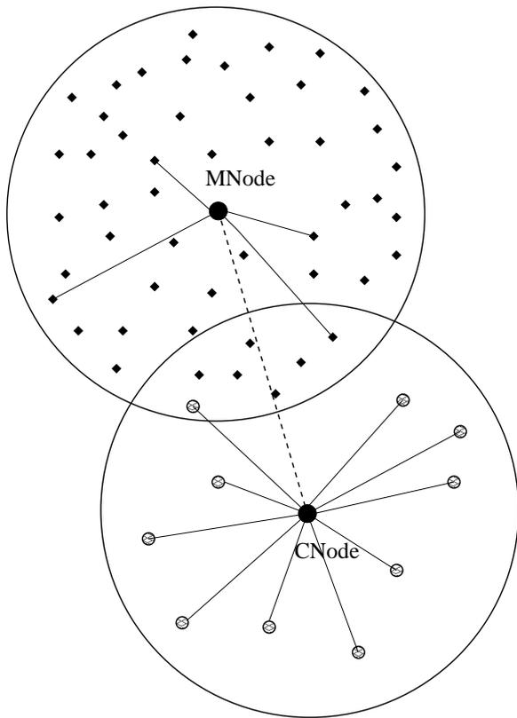
Fig. 2. The reference network, centralized in the CNode, faces the interference caused by a second UWB network, centralized in the MNode, become active in the area. The MNode is able to listen to the CNode.
