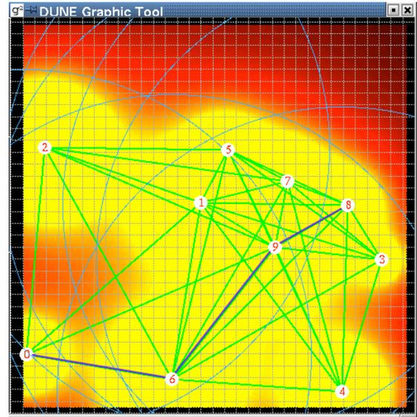
Fig. 1. Example of minimum-energy route between nodes 0 and 8, subject to high interference, especially in 9.
