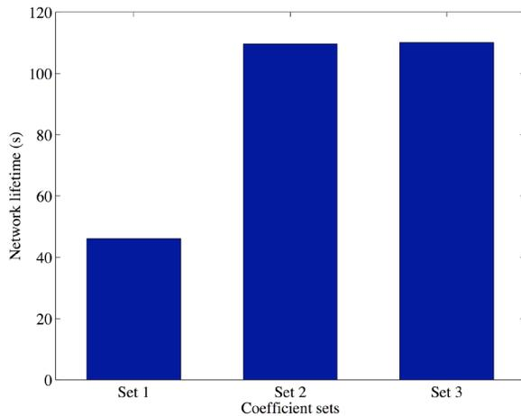
Fig. 6. Time of first node death as a function of the coefficient set in presence of external interference.
