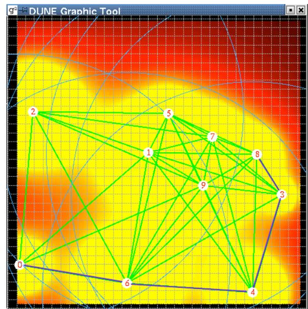
Fig. 2. Example of a topology sensitive minimum-energy route between nodes 0 and 8. Note that compared to Fig.1 this route avoids highly interfered nodes such as node 9.
