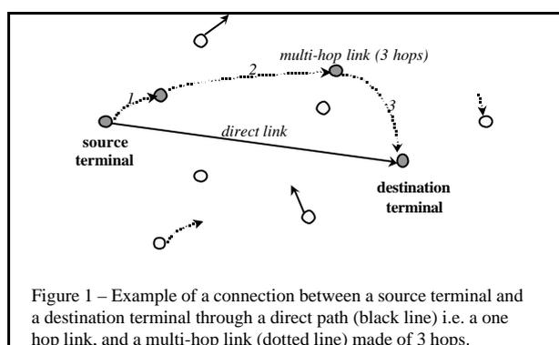
Figure 1 – Example of a connection between a source terminal and a destination terminal through a direct path (black line) i.e. a one hop link, and a multi-hop link (dotted line) made of 3 hops.
