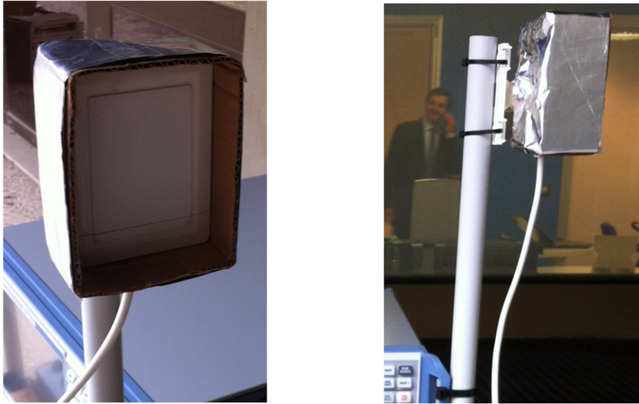
Figure 2.5: Receiving antenna modified.
