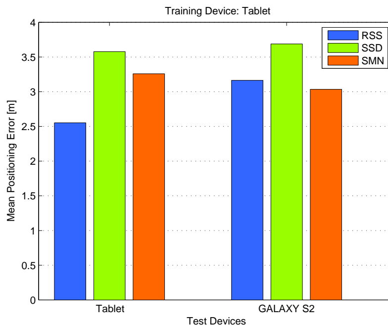
Fig. 4.9 Mean positioning errors obtained by applying the WkNN estimation algorithm with RSS, SSD, SMN methods and considering Tablet as training device.
